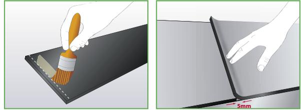
The cut sheets should be positioned so that there is a 5-10mm overlap (for compression). Do not apply adhesive to this area..
