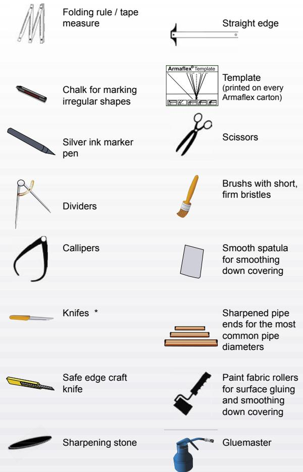
\* A three knife set plus sharpening stone are available together as a tool kit
