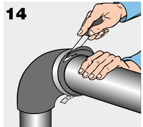
Make sure that the two sections have bonded securely on the inside as well, pressing with your fingers along the joint.
