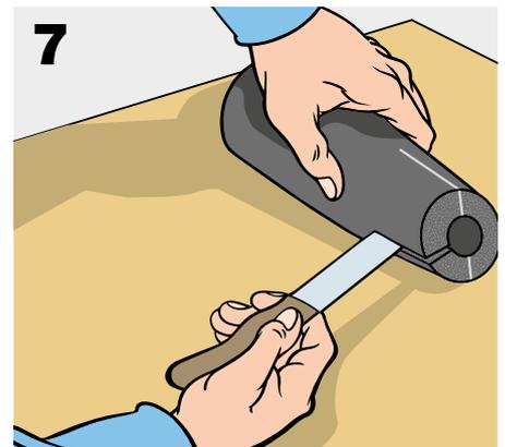
After positioning it on the pipe, glue the edges of the lengthwise cut with K-FLEX® glue and bond the edges of the sleeving to the other two sections of tubing.
