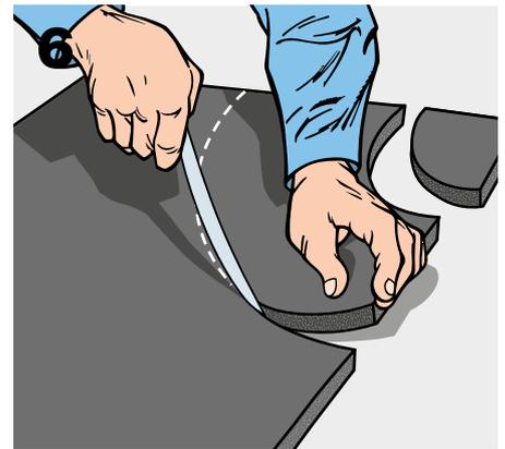
Place the section obtained on the reverse side of another sheet and use it as a template to cut out a second, mirror image section.
