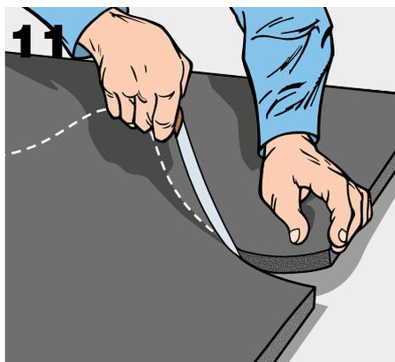
Chamfer the curved edge towards the inner surface.
