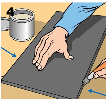
Wrap the insulation sheet around the pipe and press the glued edges together starting at the ends, then the center and then working along the rest of the length.
