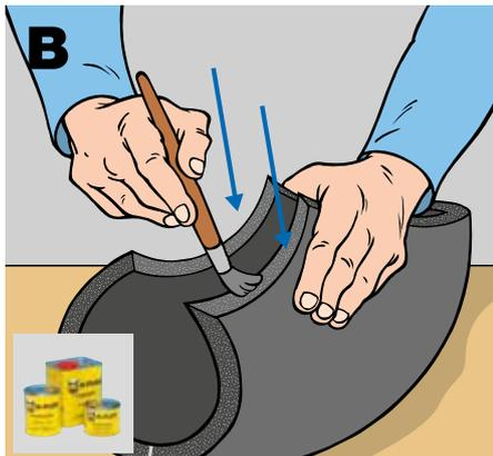
Position the K 90 piece on the bend to be lagged.
