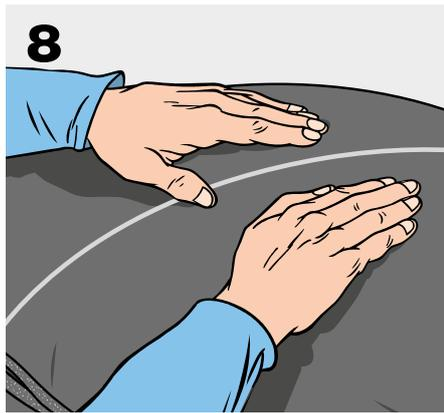
When the sheet has stuck, glue the edges all the way round.
