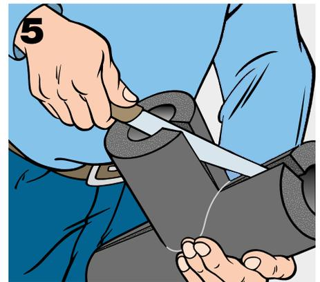
Stick the insulation to the T-junction. Then the three straight tube sections can be attached and glued together.
